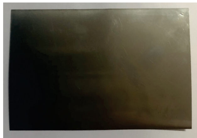
Figure 2 Test sample made of steel X6CrNiTi18-10
