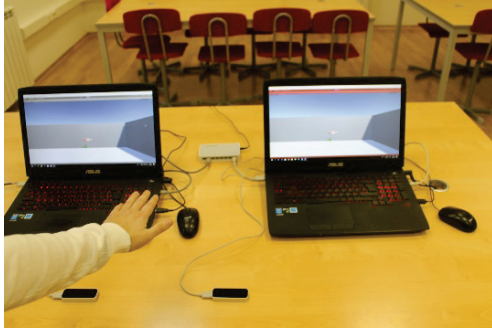
Figure 5 Hand in the middle tracked by both left and right sensor
