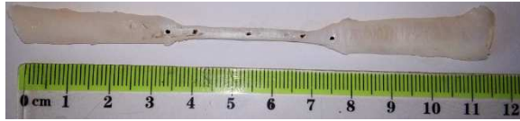
Fig. 8. The final shape of the specimen (dog-bone)
