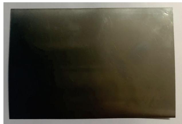
Figure 2 Test sample made of steel X6CrNiTi18-10
