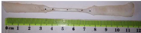
Fig. 8. The final shape of the specimen (dog-bone)
