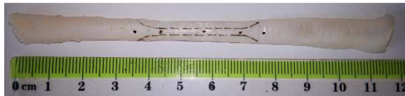
Fig. 7. Markers on the specimen
