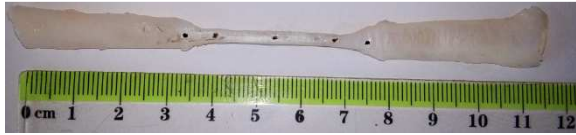
Fig. 8. The final shape of the specimen(dog-bone)
