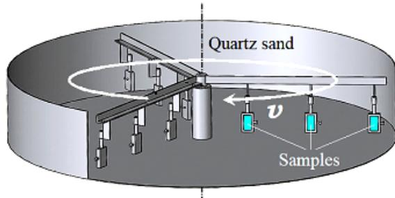
Figure 4. Schematic presentation of the wear tester
