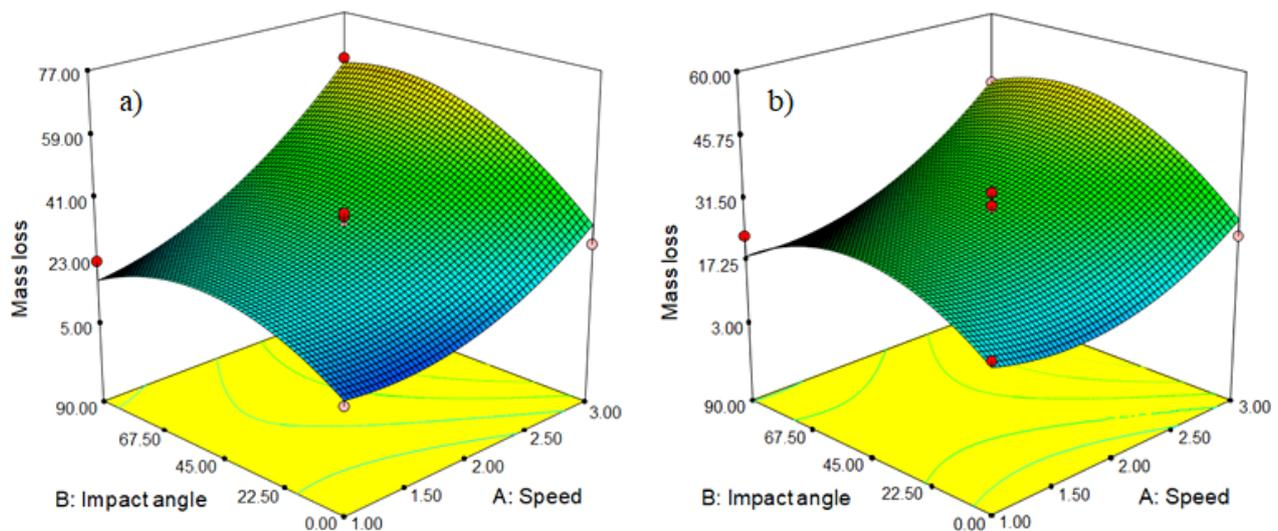
Figure 6. Response surface plots of mass loss for VC coatings – conventional (a) and duplex (b)
