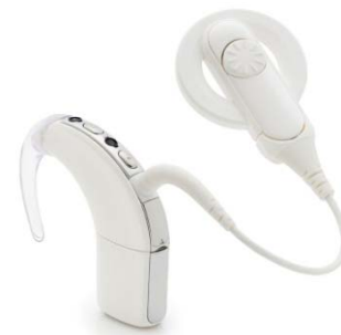
Figure 1. The external part of a CI (model The Cochlear™ Nucleus® 5 Sound Processor CP810) Picture taken from www.cochlear.com
