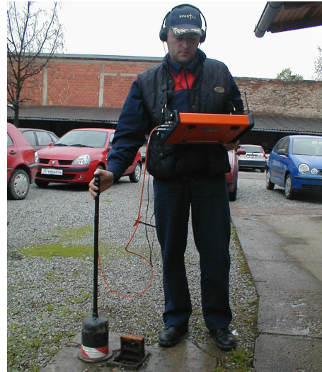
Figure 9 Measurements with Geophone
