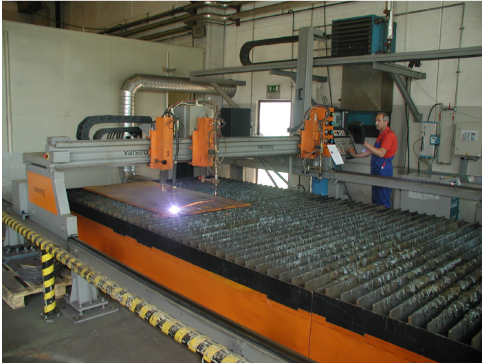
Figure 7. Modern CNC plasma cutting concept for economical industrial application
