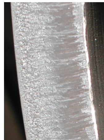
Figure 8. An example of stainless steel air plasma cutting in bellows production process. a) detail of cut surface quality b) welded cylindrical ring after air plasma cutting and cold forming process
