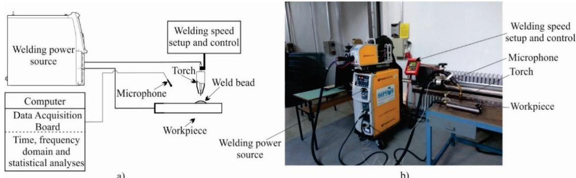
Figure 2 Experimental set-up a) schematic diagram, b) the sound measurement unit
