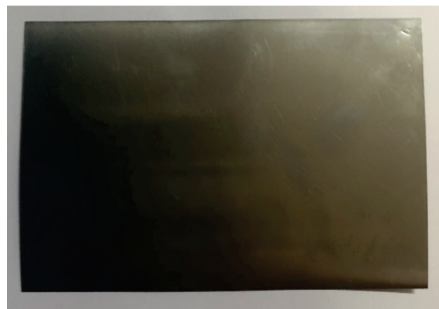
Figure 2 Test sample made of steel X6CrNiTi18-10
