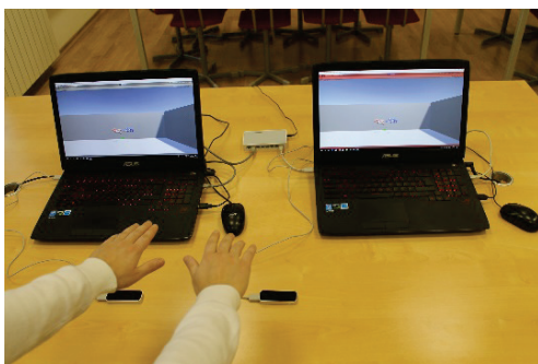
Figure 7 Two hands in the middle in FOV of both sensors – software depicts data from both local and remote sensor
