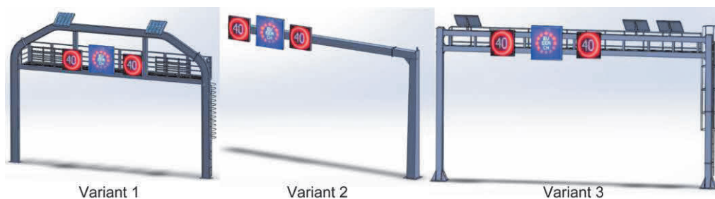
Figure 3. Conceptual variants of supporting structures
