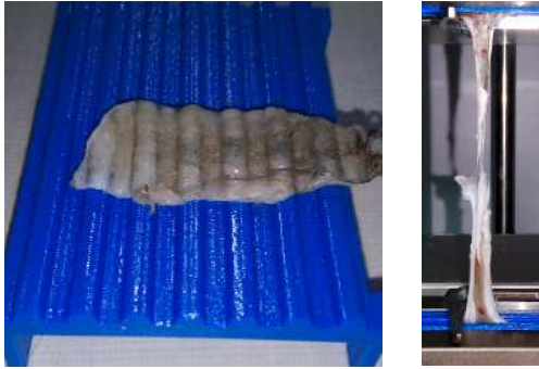
Fig. 10. Clamping area and mid-substance failure of the specimen after the tensile test
