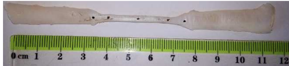
Fig. 8. The final shape of the specimen (dog-bone)
